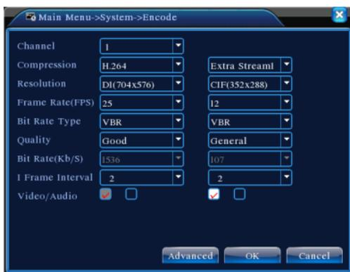
Picture 10 Encode setup
