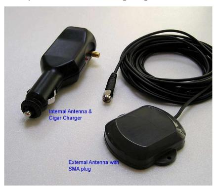
The RA-50 is a complete GPS L1 band signal re-radiating unit with dual antennas to re-transmit real-time GPS satellite outdoor receptions to an indoor environment. The re-radiating internal antenna allows multi GPS receiver users to perform On-The-Fly normal receiver performance within a closed environment, while the main GPS antenna is located on an Un-Manned outdoor location.
